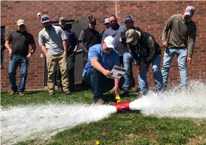
**In AFSA's Intermediate ITM Workshop, students will perform flow tests on service mains and standpipes.**
