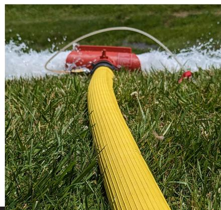
Left photo: Capti Fire pump test header set up for full flow testing. Right photo: Little Hose Monster diffusing water flow during flow testing.
